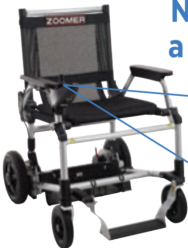
Joystick can be mounted on the right or left side for rider's comfort
